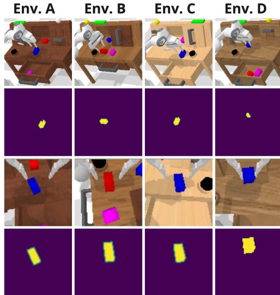
Figure 1: Overview of all four different environments in CALVIN. First row: RGB images of the static camera view. Second row: Latent representation of the static camera view of a specific object. Third row: RGB images of the gripper camera view. Fourth row: Latent representation of the gripper camera view of a specific object.
